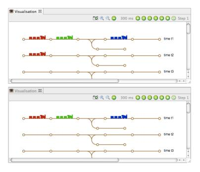
**Fig. 6.** The missing train: pictures of meet-pass at the start of a search. Propagation should deduce the position of the train at the second timestep (top picture), but in the original formulation (bottom picture) it failed to do so.
